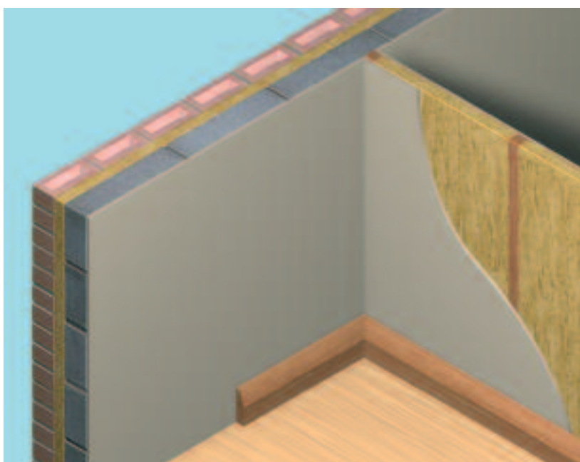
Thermal and acoustic insulation using Rockwool Slabs in floors and partitions
